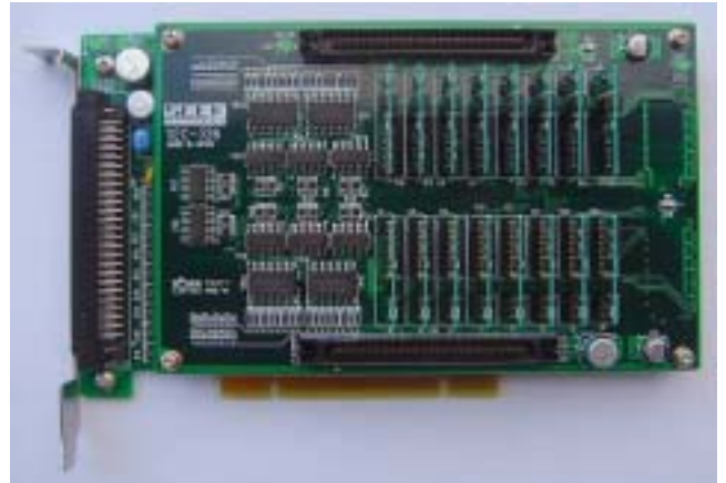
AS - FPGAPC4 - 50 汎用I/O拡張タイプ
